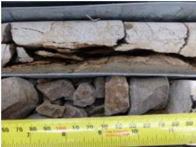
Figure 4 Thicker weathering zone along vertical joints
