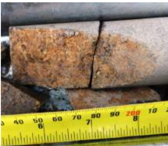
Figure 3 Thin limonitic coating on joint facing, typical for the horizontal and low angle joint sets
